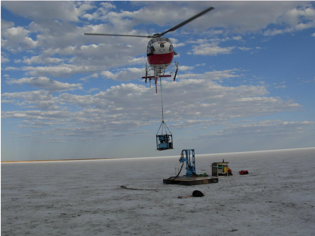
Helicopter Borne Geoprobe Rig - Lake MacKay Drilling Programme, WA
