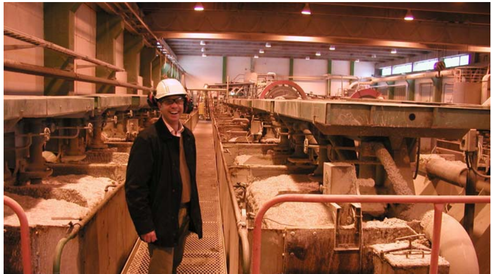
Flotation Cells
