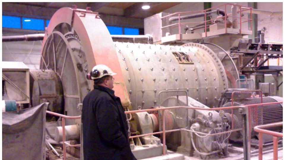
Primary Grinding Mill
