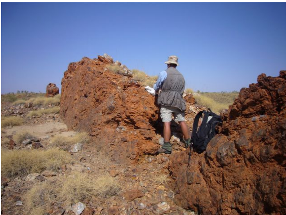
Photo shows rock chip sampling taking place on one of the better exposed veins. Here the vein is about a metre wide.
