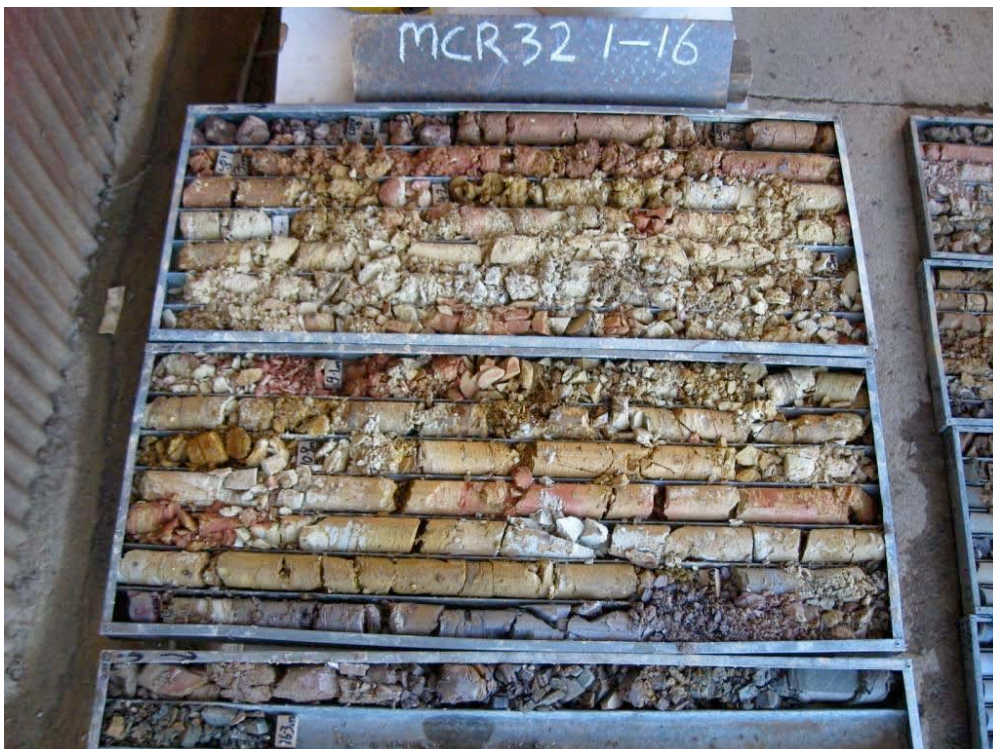
Photo 2. Drill core from Hole MCR 32, showing extreme alteration of rocks to swelling clays, overlying basement.
