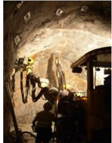
The Sons of Freedom reef was intersected in 2006 during construction of the upper part of the Warrior decline. The long exposure of the vein for some 50 metres, along the side and across the face of the Decline, yielded valuable information on its gold content and potential for mining. Channel sampling of the quartz and sulphide vein in this location returned 0.2 metres true width at 362 g/t Au (11.6 ounces per tonne), equivalent to 36 g/t Au over a two metre mineable width.
