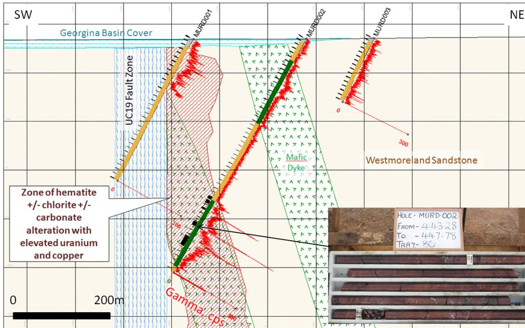
*Fig.1. Cross section showing interpreted geology and gamma log results from the UC19 area. Black regions on the drill traces show areas sampled for the previously reported set of results. The entire interval from 385 metres to 542 metres has now been sampled.*
