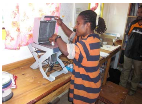
Niton XRF Analyser in operation at Yandera
