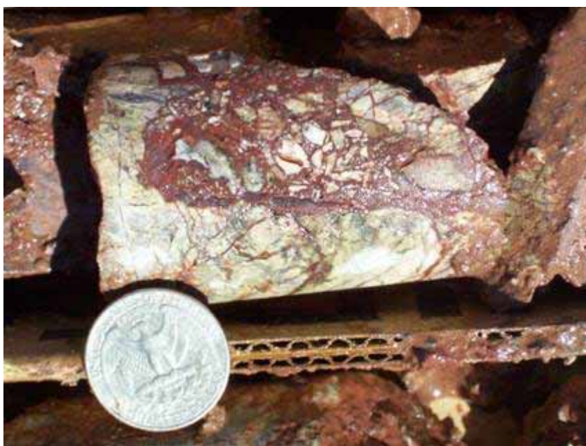
FIGURE 11: CORE FROM THE BERNARD DRILLING SHOWING BRECCIATED “LOWER PLATE” ROCKS WITH HEMATITE AND QUARTZ VEINING
