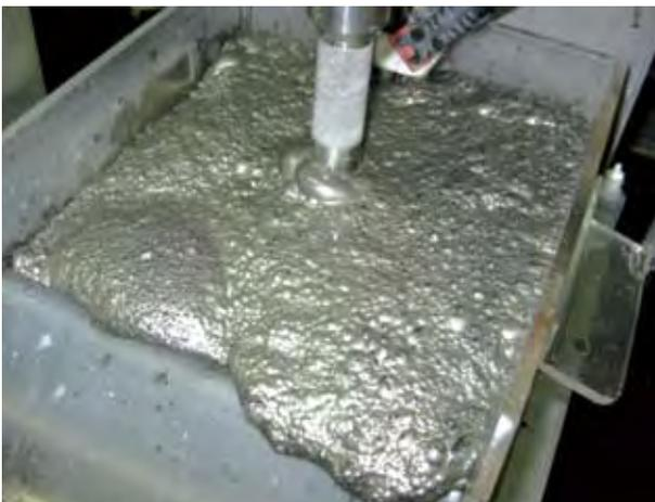
Flotation test work on Savoyardy ore.
