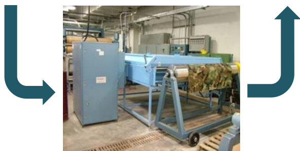
RST PROCESS: Low energy microwave treatment
