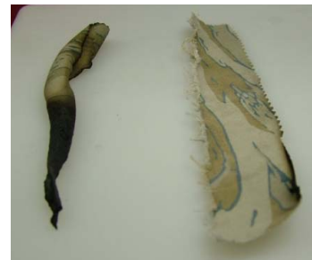
Untreated fabric (left) vs. RST treated flame retardant (right)
