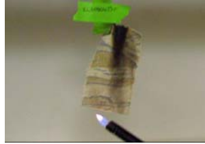
Alexium's flame retardant textiles are self extinguishing
