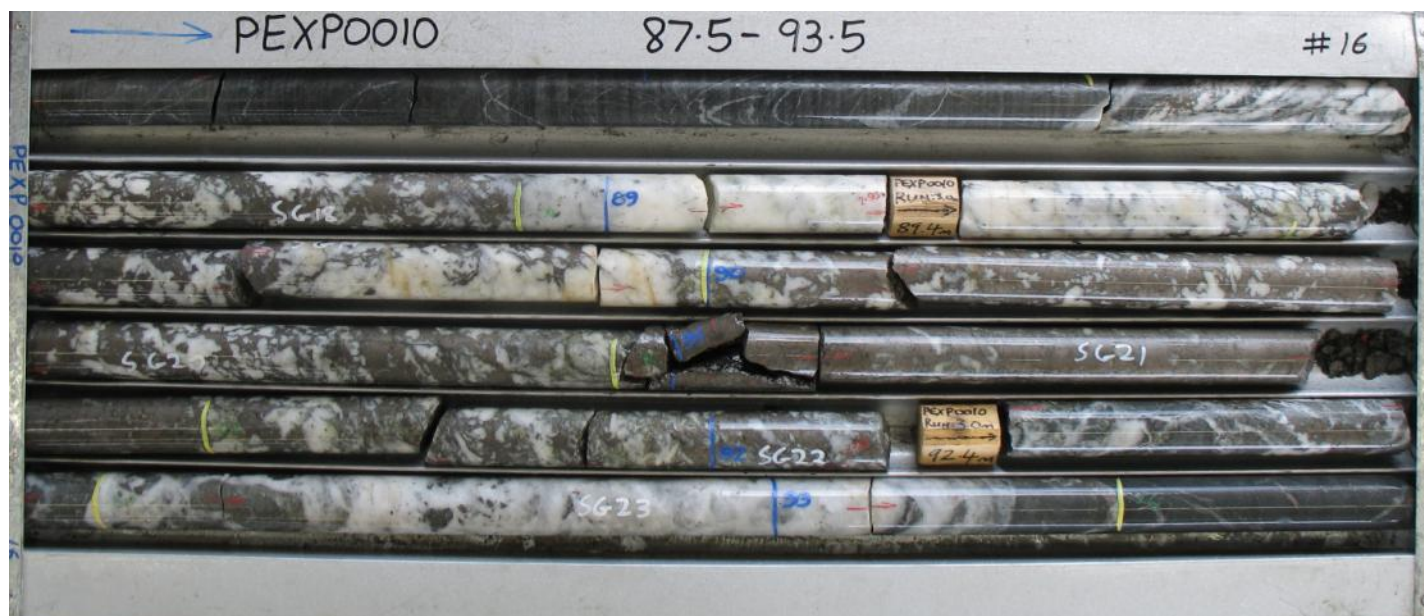
Figure 2 - High-grade Perseverance intersection (4.93m @ 31.66g/t)
