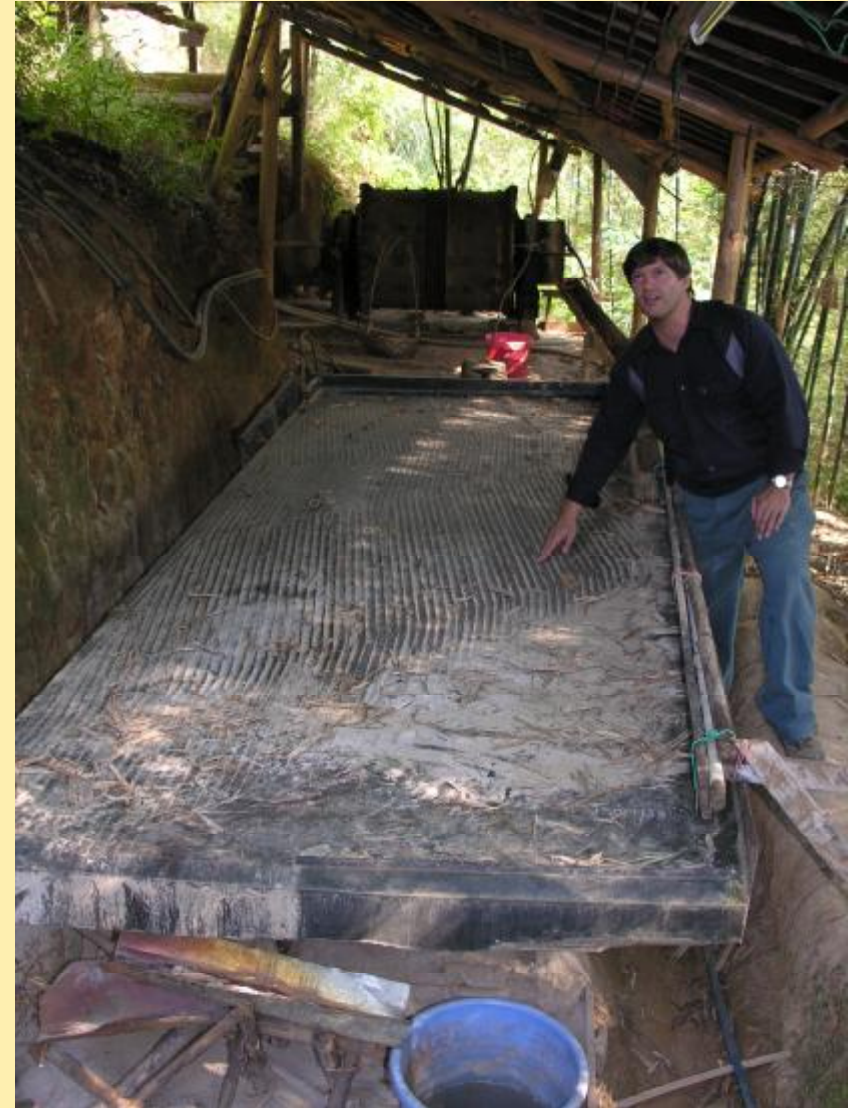
Gravity separation table at Teningding for concentrating heavy minerals and visible gold.
