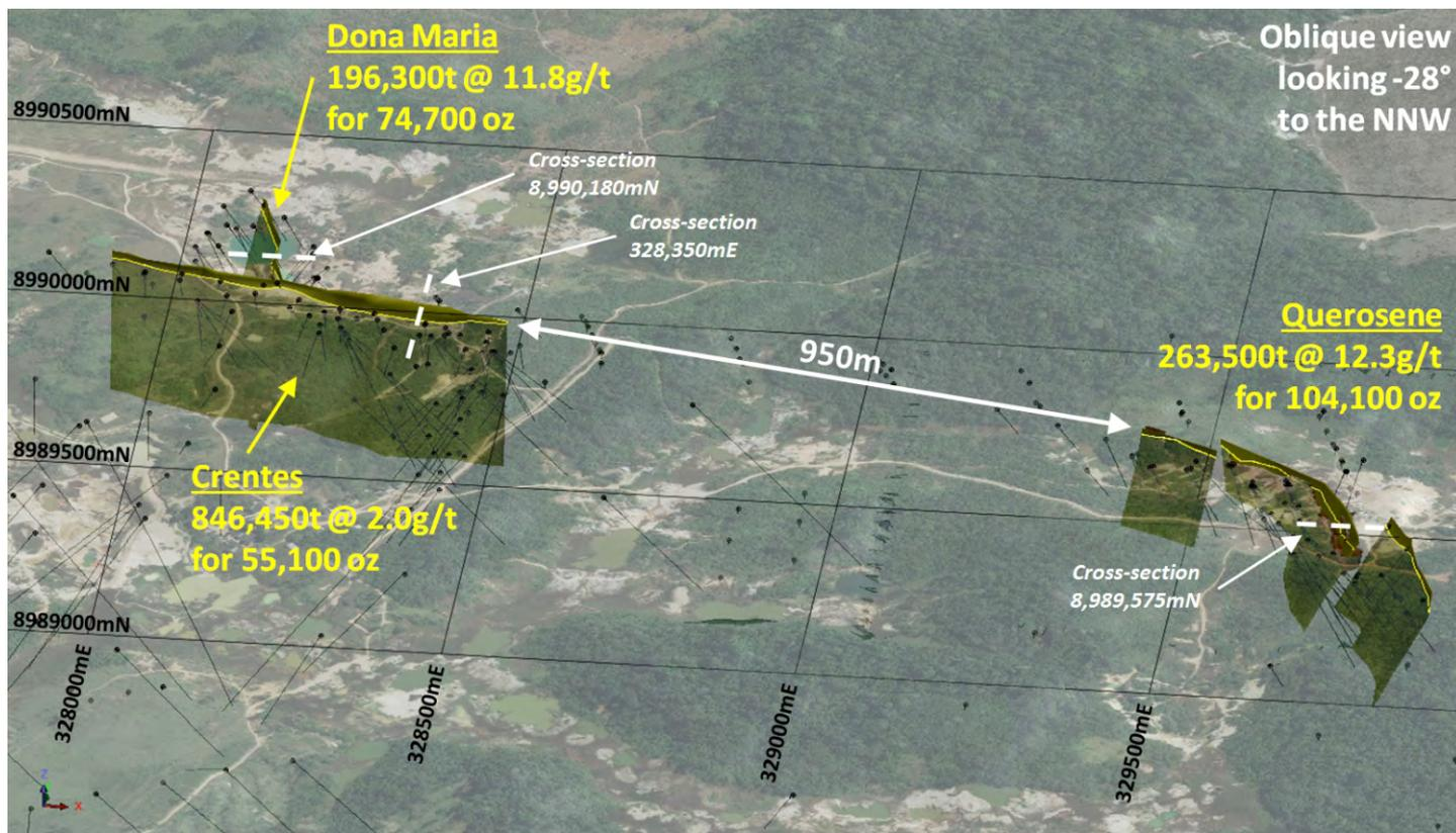
QUEROSENE RESOURCE MODEL SHOWING PRELIMINARY MINE PLAN - LOOKING DOWN TO NE
