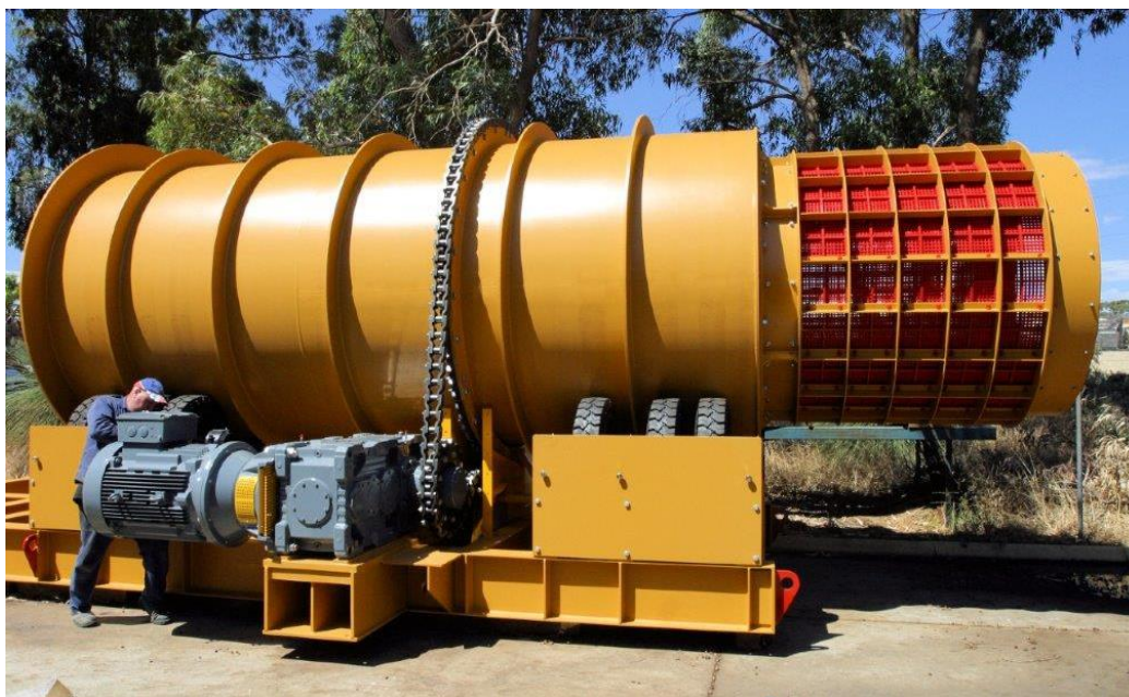
Figure 1. A scrubber of the type that would be used for the Malingunde saprolite-hosted flake graphite deposit in a production scenario.
