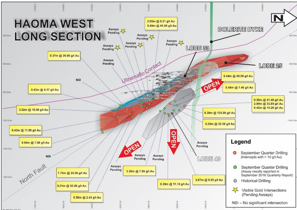
Figure 7: Long section showing the Haoma West Lode 25, Lode 33 and Lode 40 resource outlines with drilling results.
