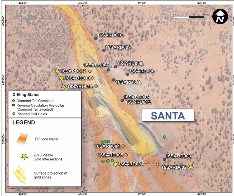
Figure 10: Plan view showing the Santa host BIF unit and the locations of drill holes.
