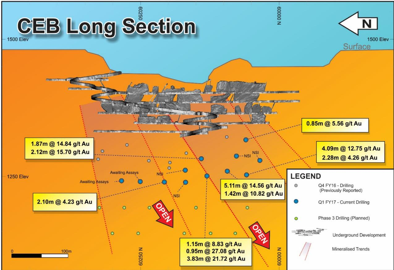
Figure 12: Long Section view of Cock-eyed Bob showing decline development, ore drives, and drilling results.
