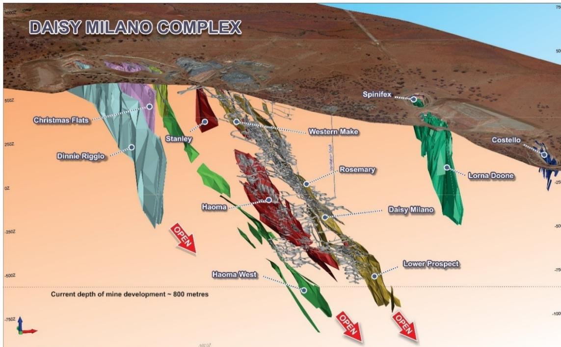
Figure 5: Schematic view showing the mines that make up the Daisy Complex.
