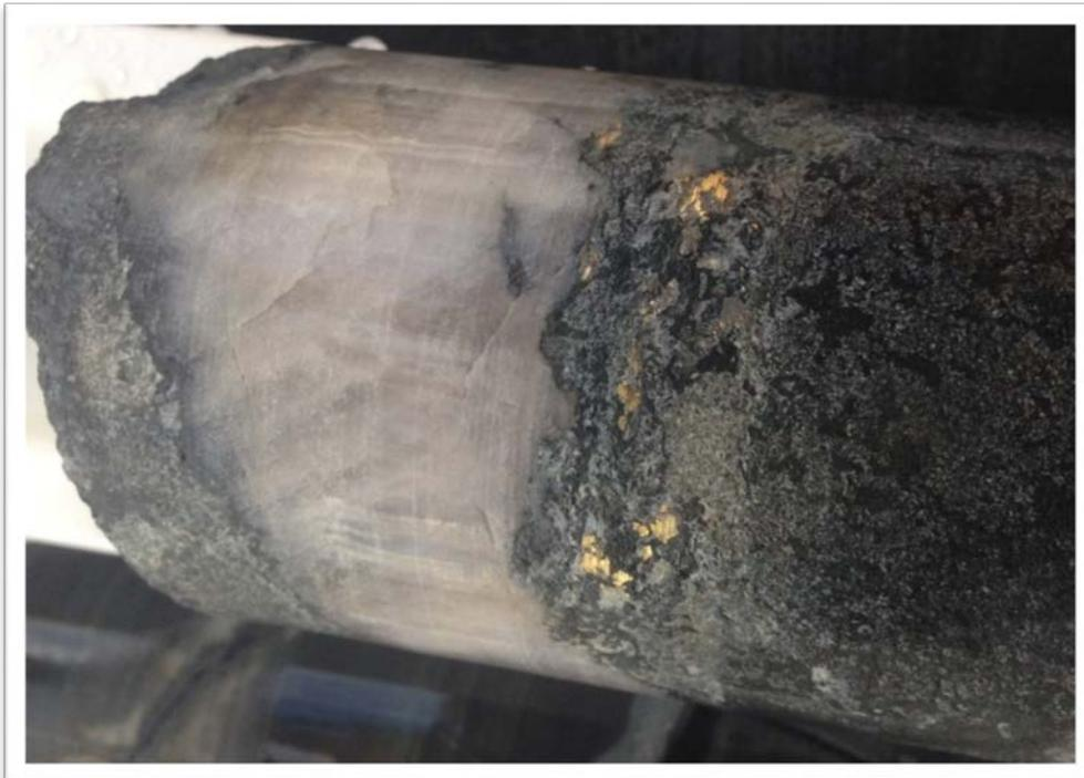
Figure 11: Spectacular Visible Gold intersection in diamond core at 155 metres down hole in 16SARD012. Width of the HQ diamond core is 63.5mm.
