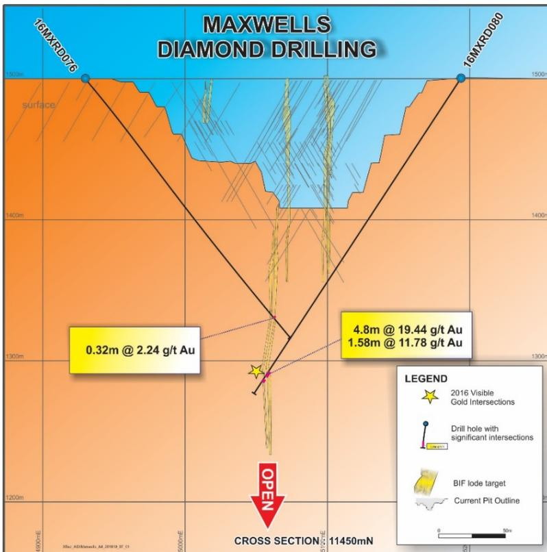
Figure 9: Maxwells drilling cross section 11450mN.
