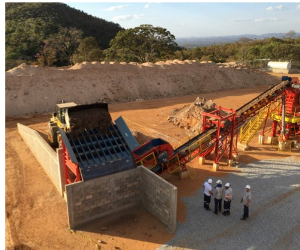
Commissioning Material on the conveyors of the crushing circuit.
