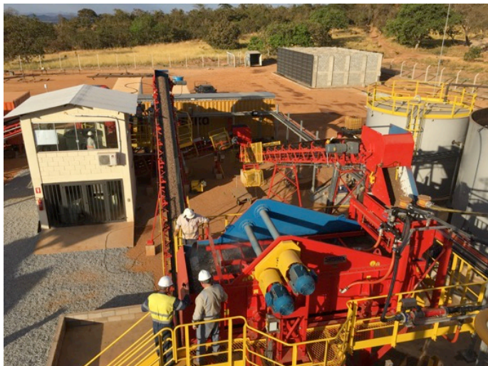
Commissioning Material on the conveyors of the crushing circuit.
