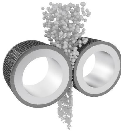
The rollers are studded, which assists in forming an autogenous layer of ore on the surface of the rolls, thereby crushing ore-on-ore, realising exceptional wear life and high comminution power efficiency (see Figure 2 below).
