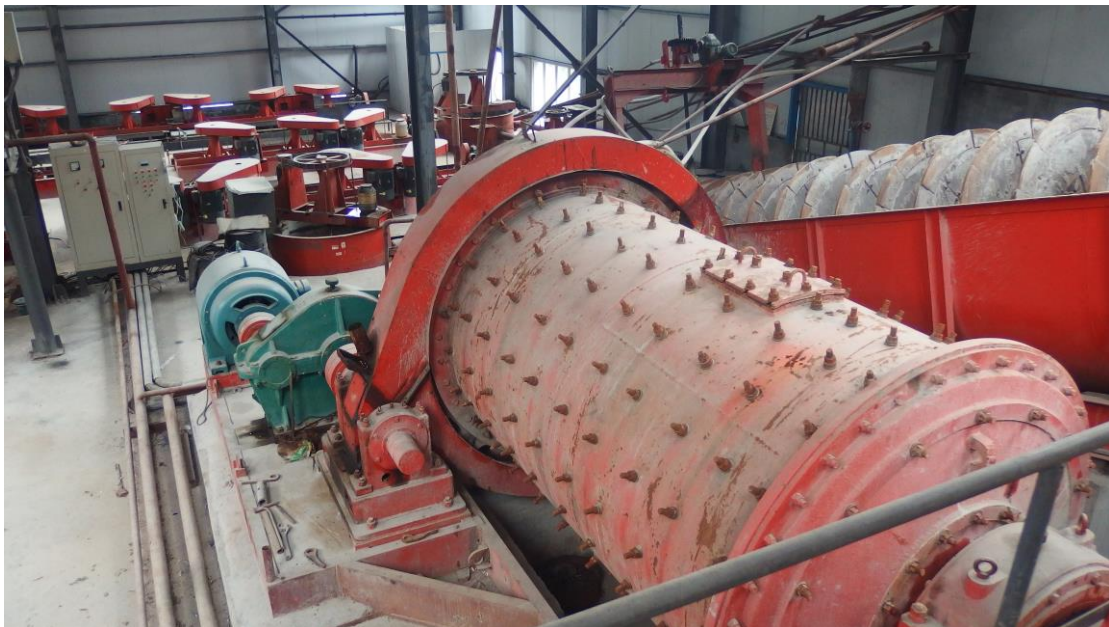
Figure 4-7 Ball mill crusher and floatation circuit.
