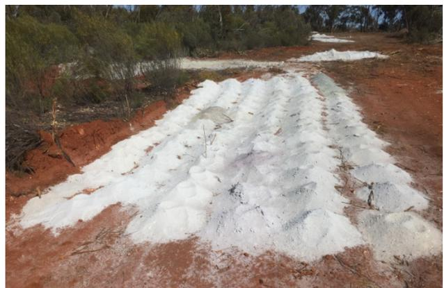
**Photograph 2.** Drill hole PD015 reached a depth of 108m, and show 103 x 1m sample piles of white pegmatite.
