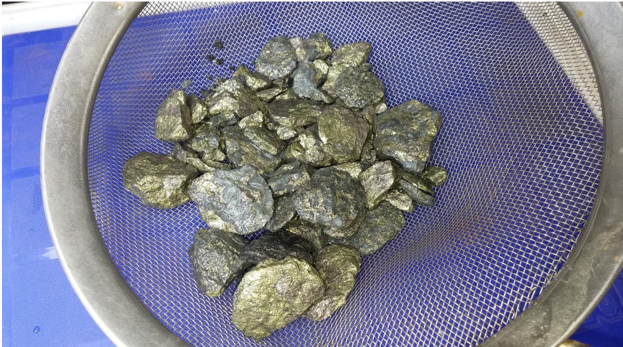
**Figure 7 Sieved chips from drill hole AKC006 79-80m showing coarse chalcopyrite with pyrrhotite and pentlandite**
