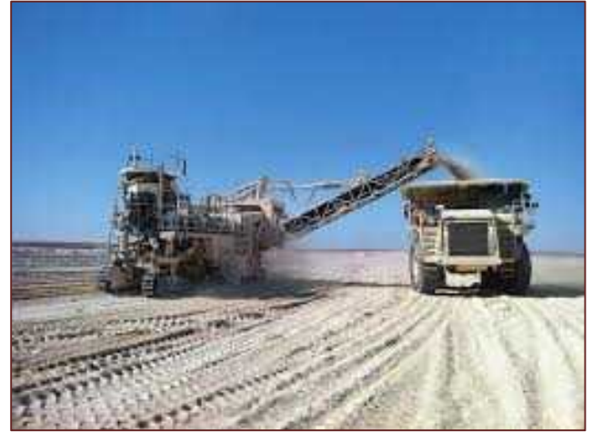
Photo: Surface miner loading haul truck
