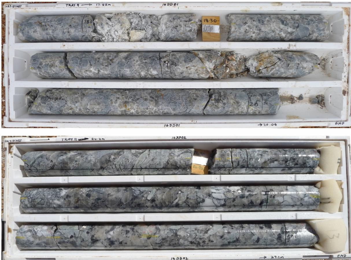
Figure 3: Examples from spodumene-rich zones in diamond core at Lynas Find: metallurgical test-work and analysis of the core for lithium is currently under way. Pegmatite was intersected from 0.5 to 51.90m in 16DD01, and 16.77 to 44.00m in 16DD02.
