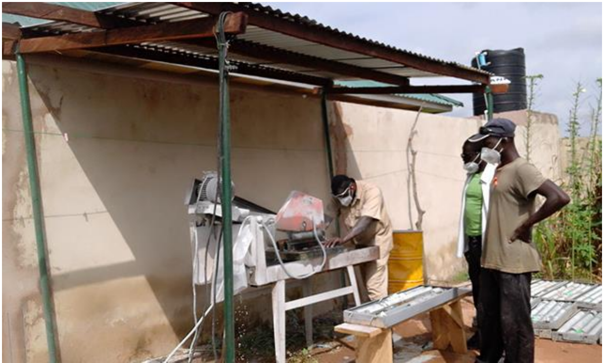
Cutting diamond core from drilling on the Kollo trend.
