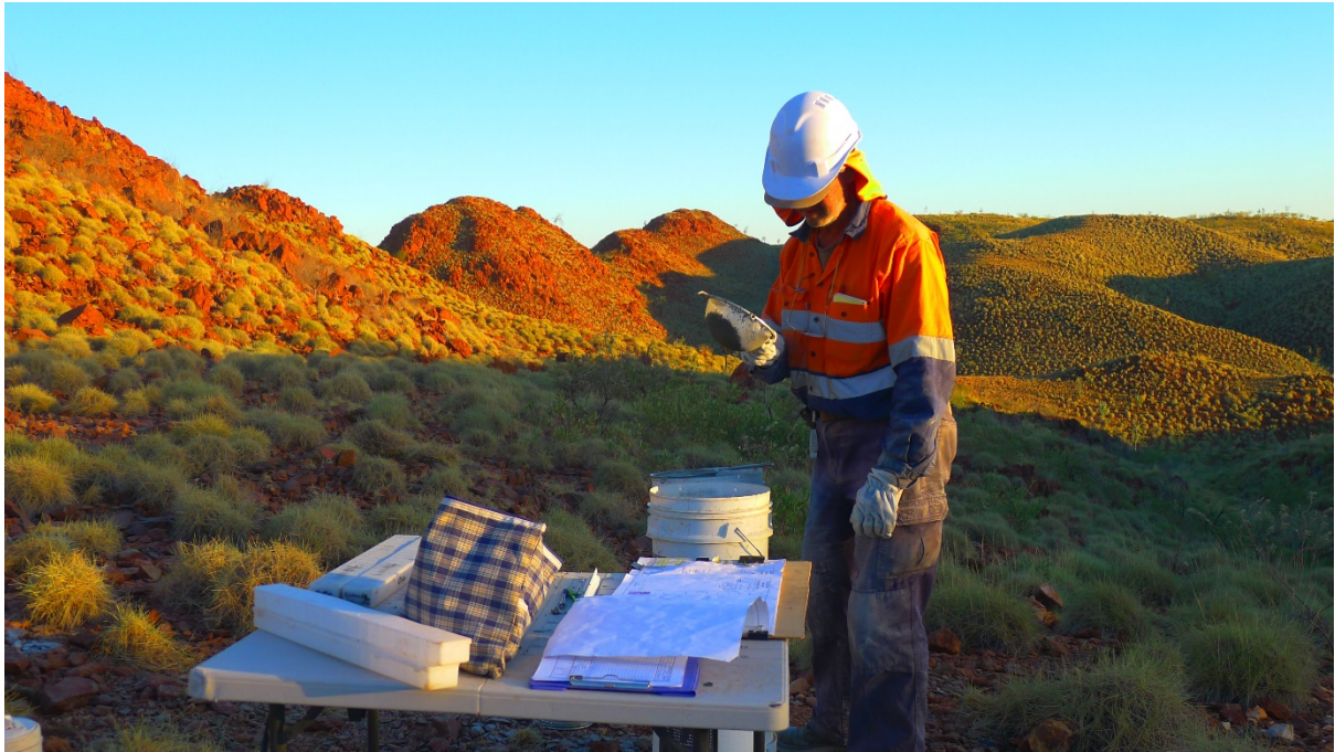
Figure 1: Logging of reverse circulation (RC) drill chips at Lynas Find
