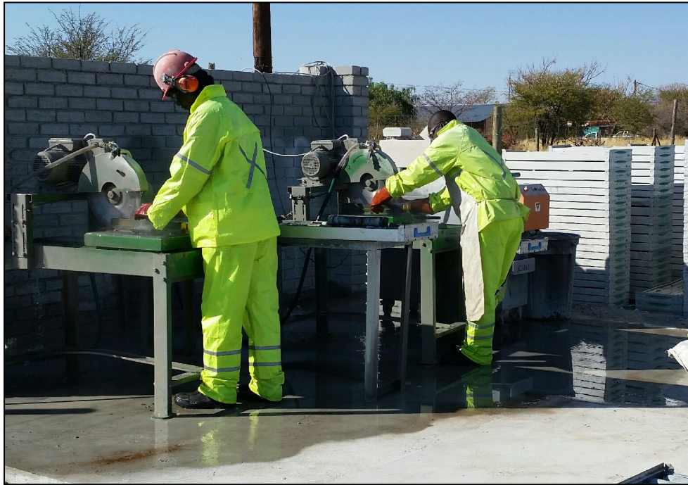
Figure 2: Cutting mineralized drill core at MOD's recently upgraded core processing facility in Ghanzi. A third core saw has been added to keep up with the rapid rate of diamond drilling at T3.
