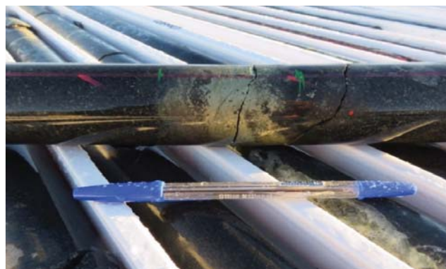
FIGURE 2. Stringer chalcopyrite (2.02% Cu) at 614m.
