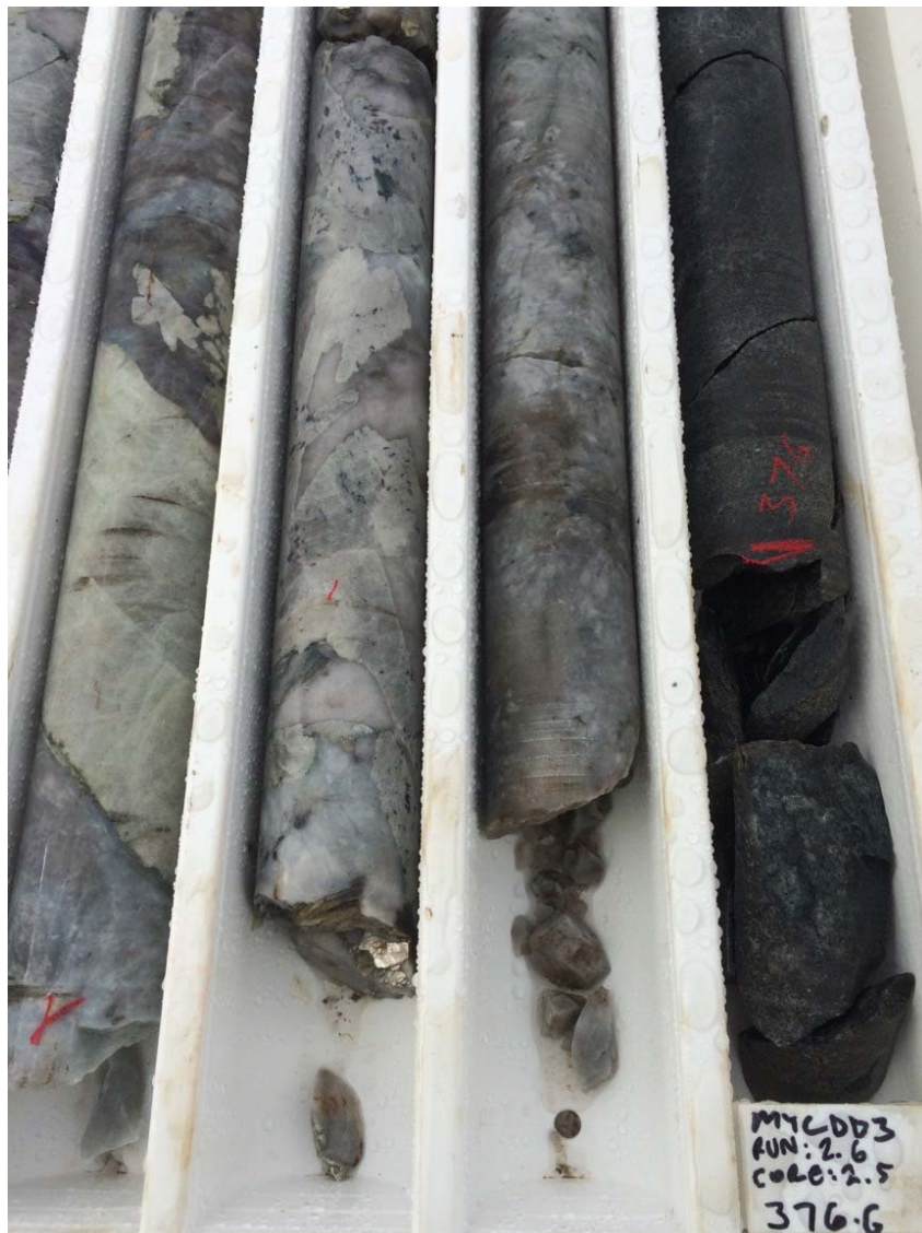
Figure 1: Coarse-grained spodumene crystals in pegmatite, intersection in NQ drill core, Hole MTCDD3, depth approx. 379m
