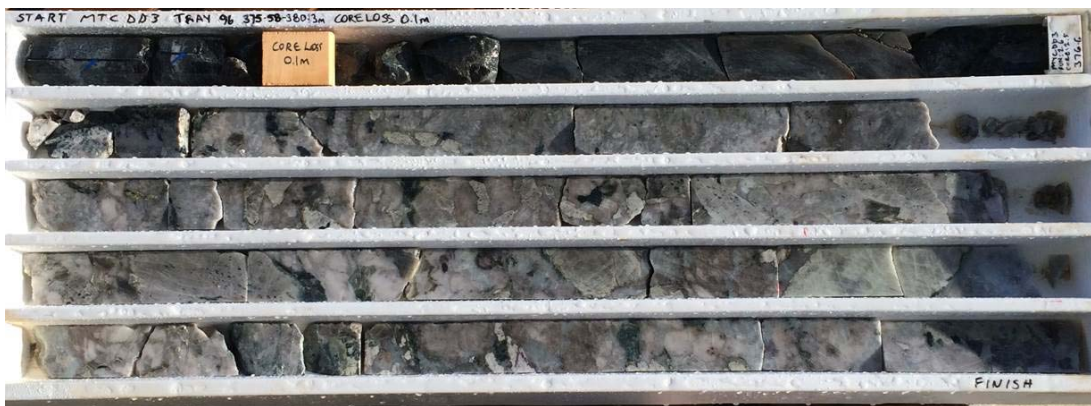
Figure 2: Pegmatite intersection in cut NQ drill core, Hole MTCDD3, depth approx. 376m, with abundant coarse spodumene crystals
