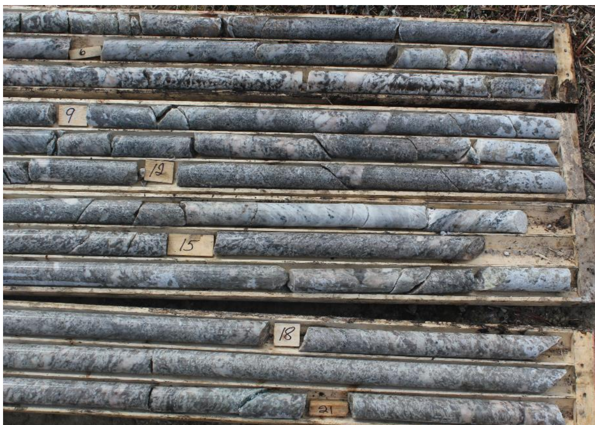
Figure 1. Drill core from the Root Lake Project showing multiple intersections of spodumene mineralisation in the pegmatite structures.
