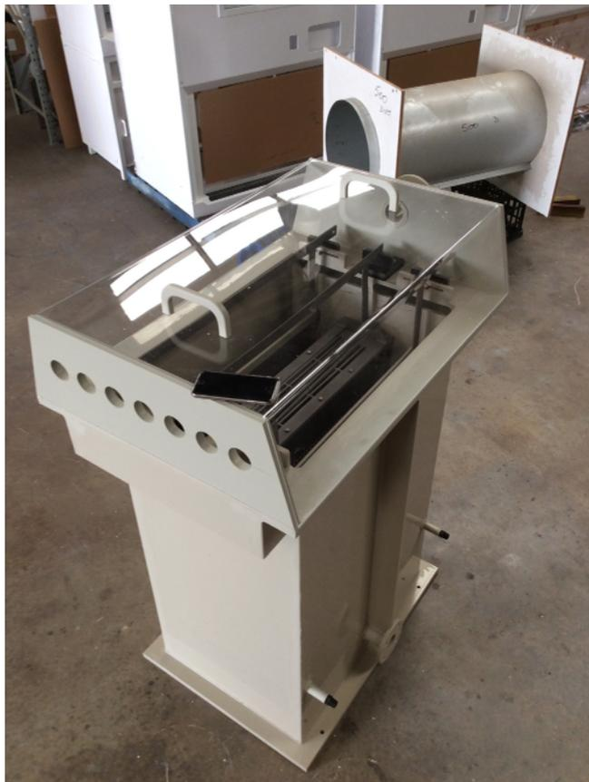
Figure 2: Cell capable of producing 5 tonnes p.a. of high quality graphene
