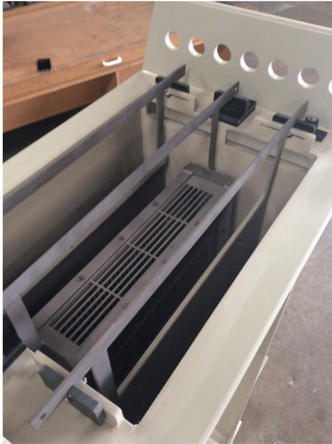
Figure 1: 250 litre production cell under construction
