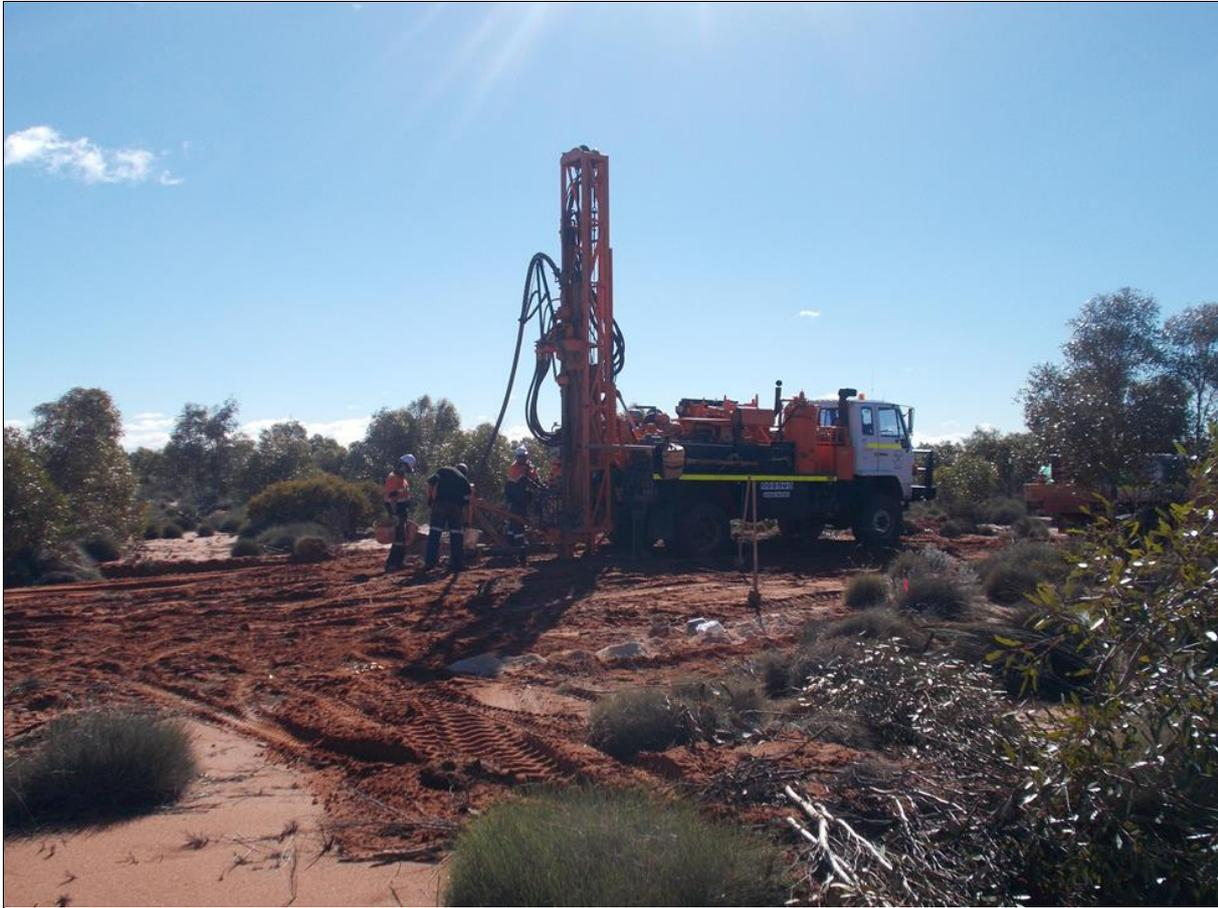
**Figure 2: Aircore drill rig at the Plumridge Gold Project**
