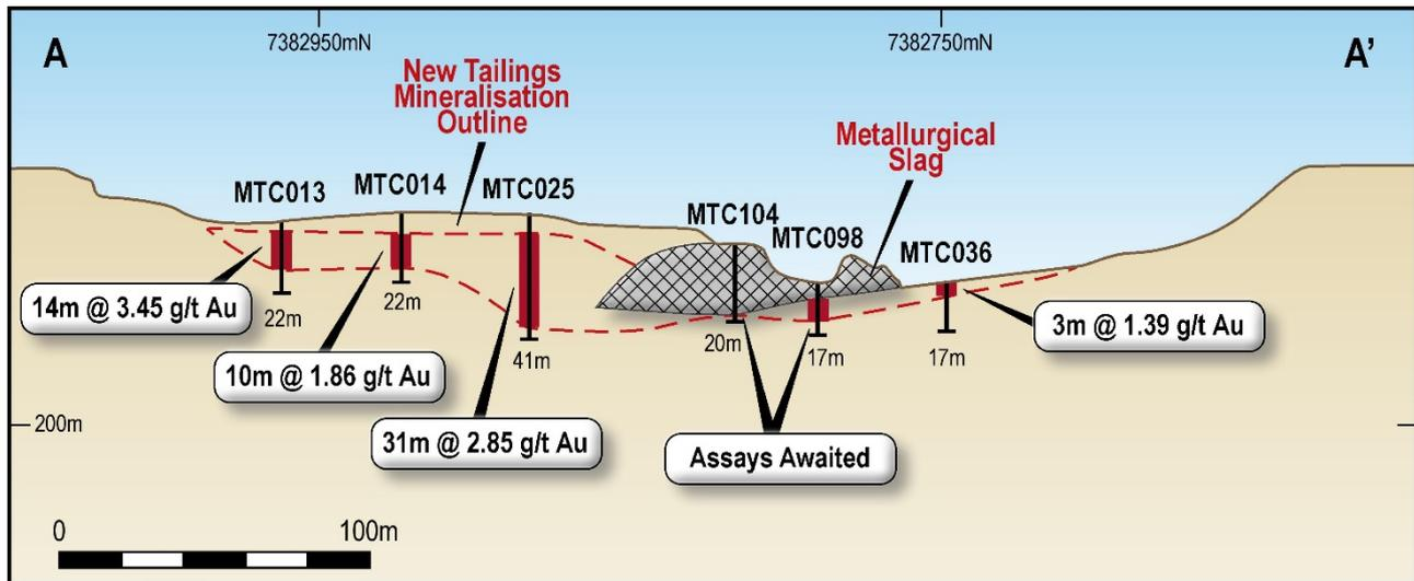
**Figure 3: Cross Section 232100E (A-A') at Mundic Gully tailings dump showing additional tailings mineralisation outside of the current Mineral Resource Boundary.**
