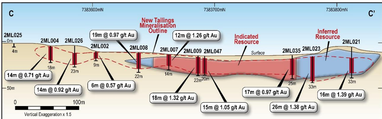
**Figure 5: Oblique Cross Section (C-C') at No2 Mill Tailings showing the additional mineralisation intersected to the southwest (left of page) of the current Mineral Resource boundary.**
