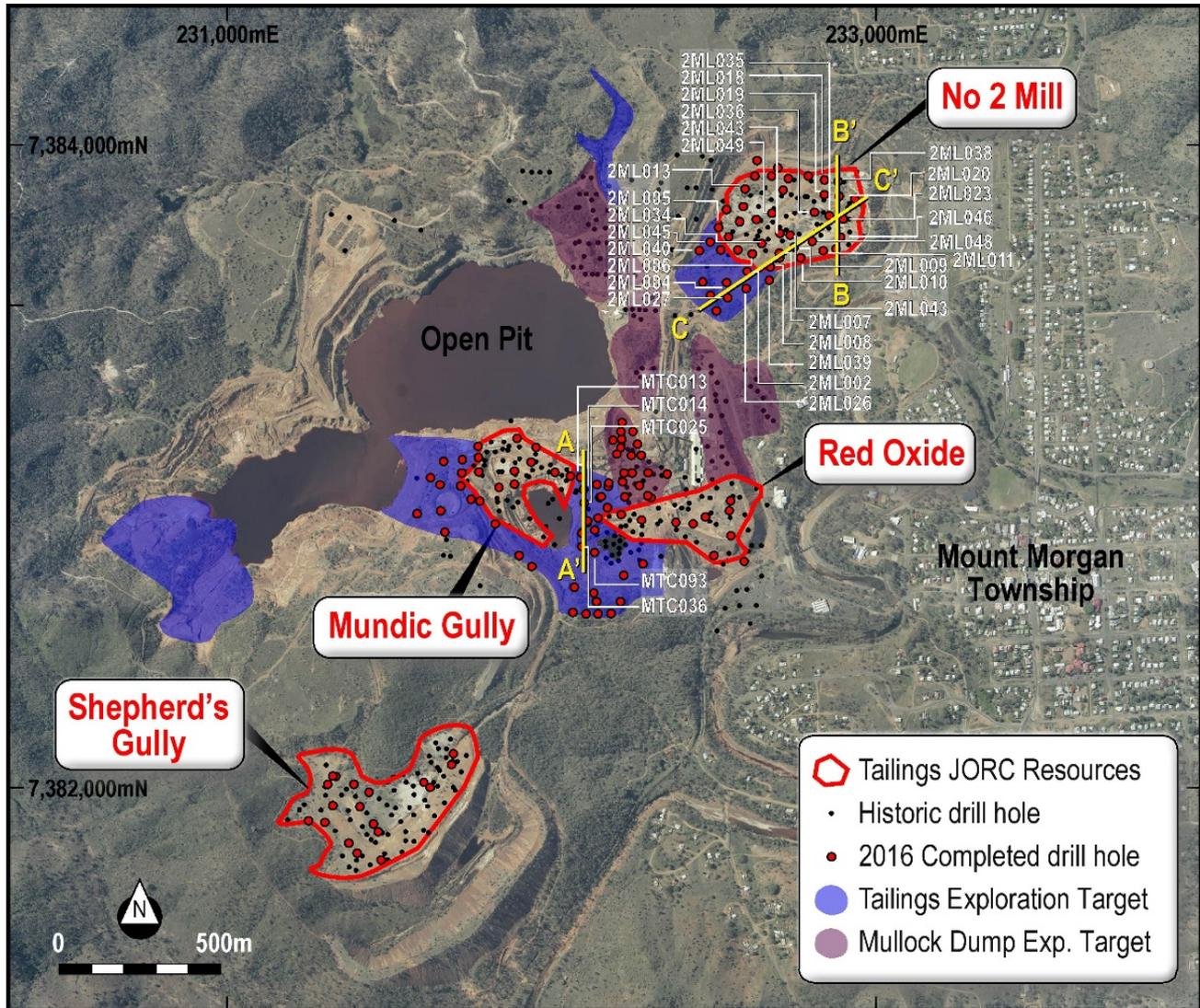
Figure 2: Completed drill holes at Mount Morgan indicating drill holes with recent assay results received (Plan view with cross section references A-A', B-B' and C-C')
