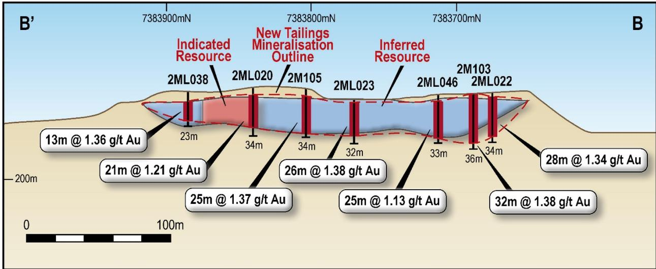
**Figure 4: Cross Section 232900E (B-B') at No2 Mill Tailings showing the consistency of the mineralisation intersected within the Inferred Resource Boundary at marginally higher grades in this drilling compared with the reported Inferred Resource Grade of 1.17g/t (Table 1).**
