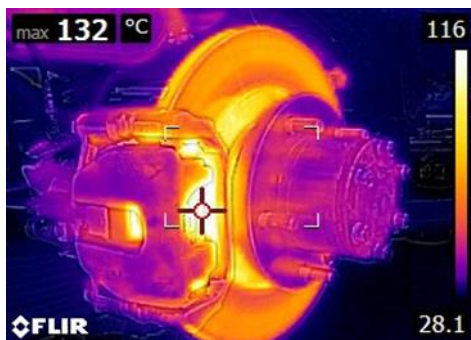
Max heat generated 132 c Polymer can withstand 300c+
