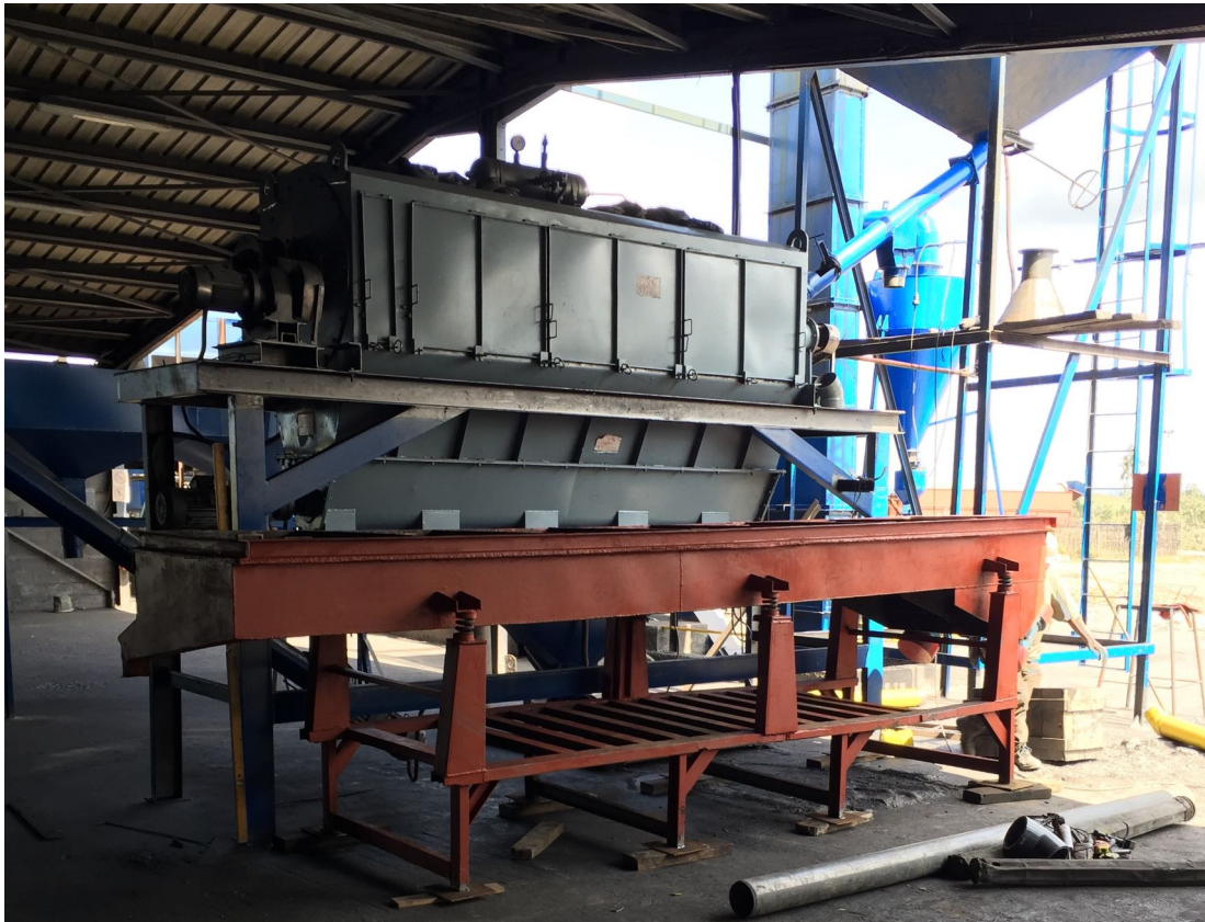
Vibrating magnetic separator being installed at Graphmada
