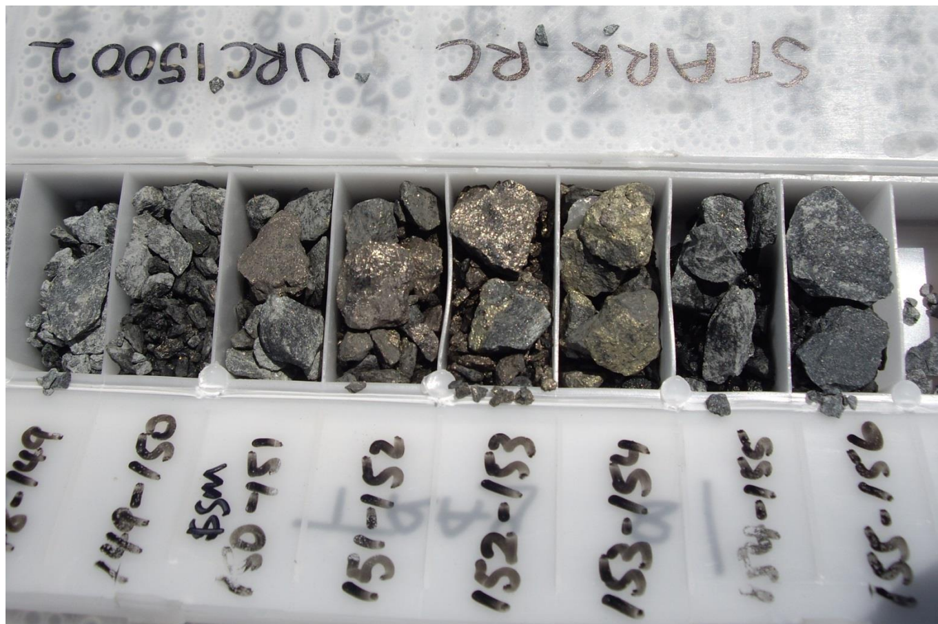
Figure 3: Photo of NRC15002 RC chip tray showing semi-massive and massive sulphides from 150 – 154 metres. Refer to Table 1 for individual copper-nickel-PGE assay values.
