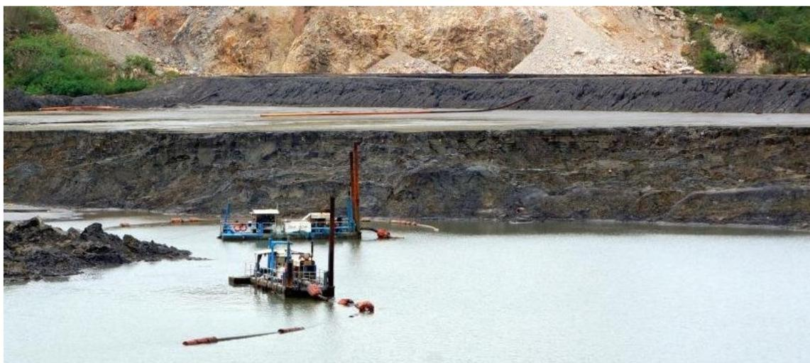
Dredging is now in coarse higher grade material which should be typical for the balance of the resource.
