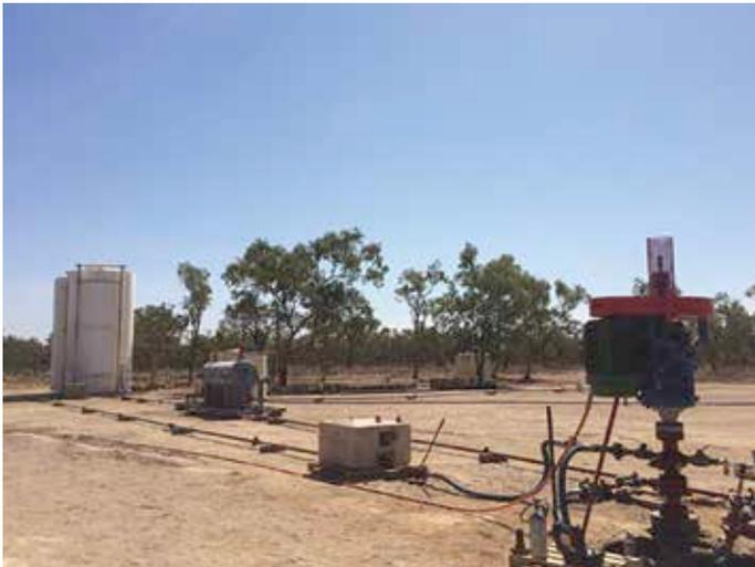
**Figure 4: Egilabria 2 well – Well and flow test apparatus.**
