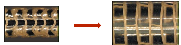
Polymer enables expansion to 4.0mm without fracture
