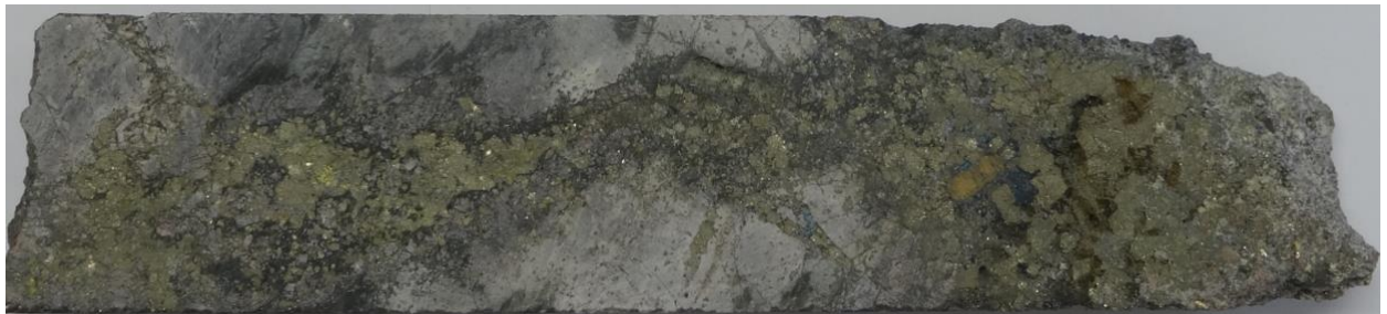
Figure 5 Chalcopyrite (pale yellow) and pyrite (yellow) veins in silicified and carbonate altered black slate host (width of core photo is 45mm)
