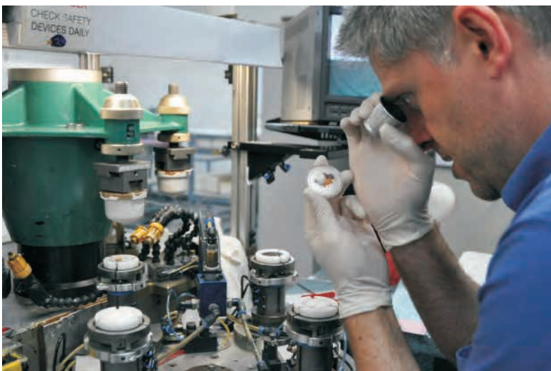
Examining the registration of a coin's printed image.
