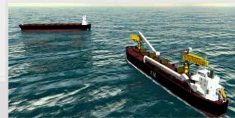
Dual conveyors and loading booms allow for rapid unloading, increasing capacity of the port
