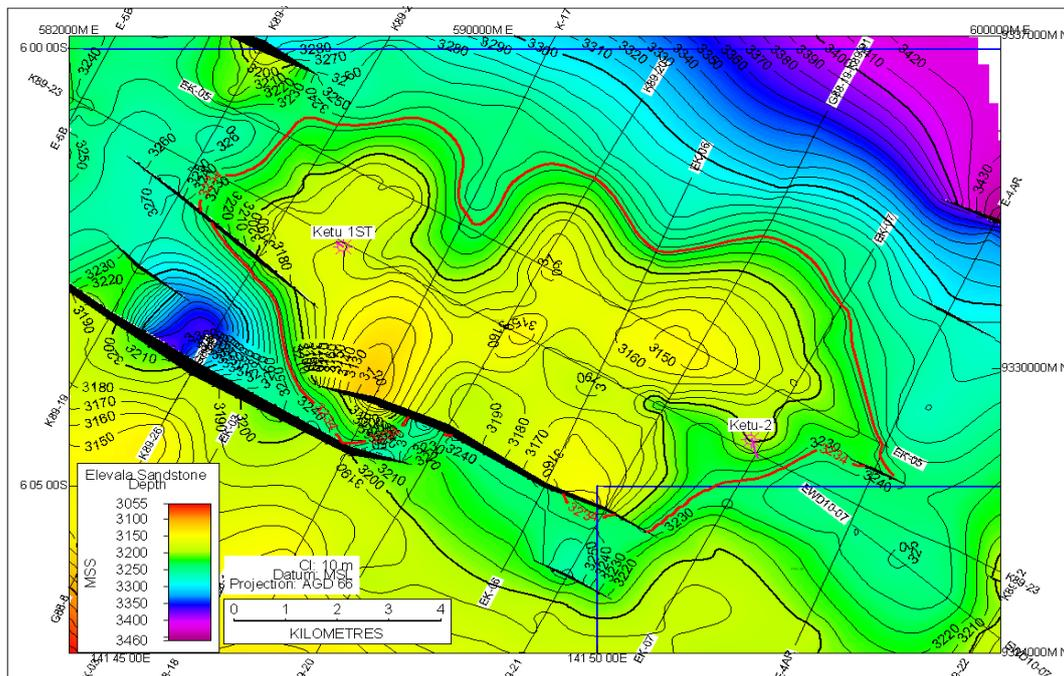
Figure 8-6 Ketu Field Elevala Reservoir Depth Structure Map
