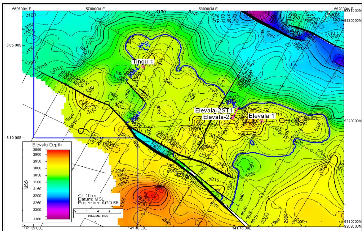
Figure 8-5 Eevala Field Eevala Reservoir Depth Structure Map
