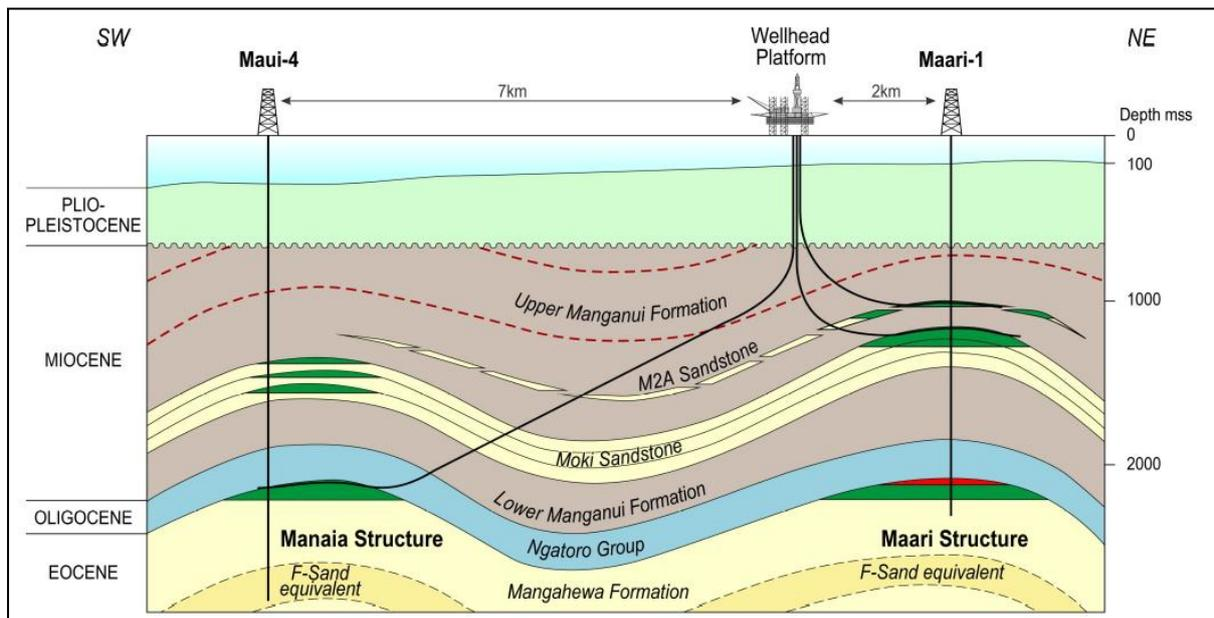
**Figure 6-2 Maari Manaia Structural Section (from Horizon)**
