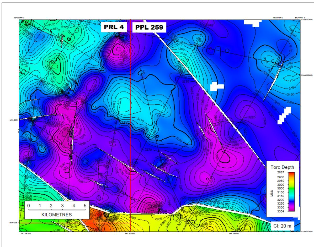
**Figure 8-13 PPL 259 Nama Prospect Toro Depth Structure Map**
