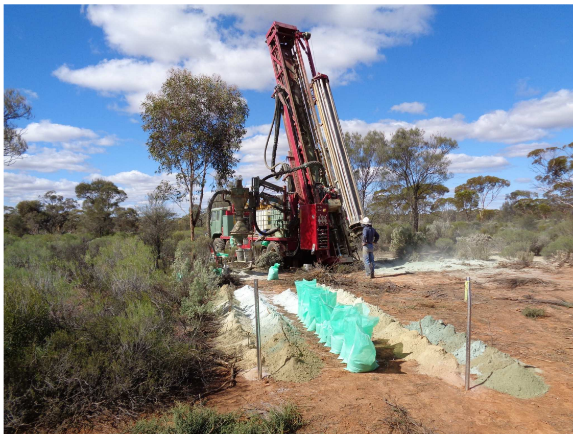
Picture 2. RC Drilling Rig type to be used at MELP for maiden drill program.
