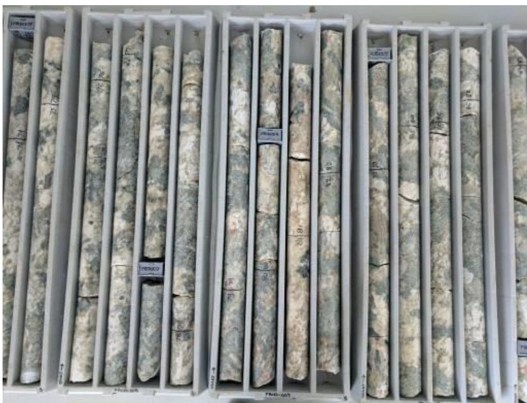
Figure 3. Large green spodumene crystals making up a high proportion of pegmatite volume hosted by lighter coloured quartz and feldspar (albite) 73.8m – 87.1m FRDD003 (HQ) Grants Prospect, Finniss Lithium Project, NT.
