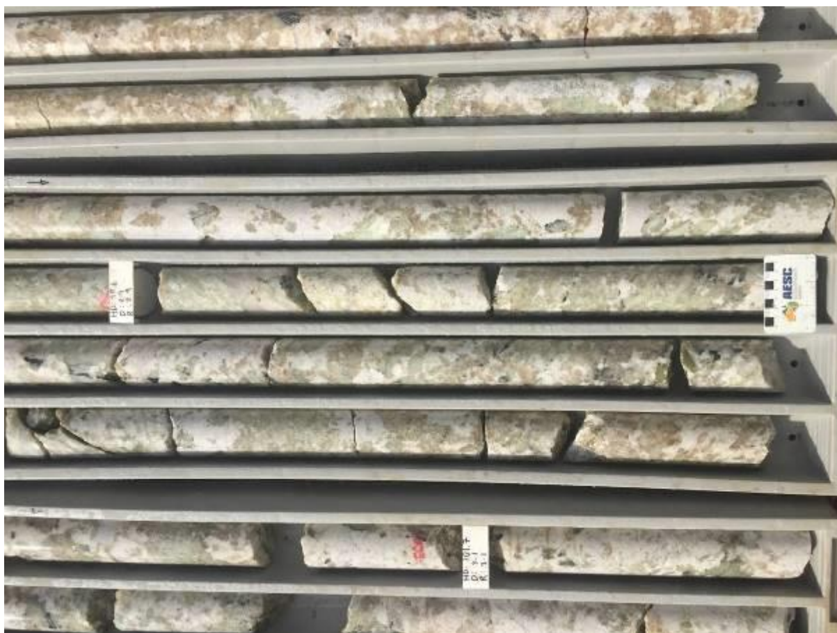
Figure 7. Light green spodumene crystals hosted by lighter coloured quartz and feldspar, 95.2m – 103.1m FRDD001 (HQ), BP33 Prospect, Finniss Lithium Project NT.
