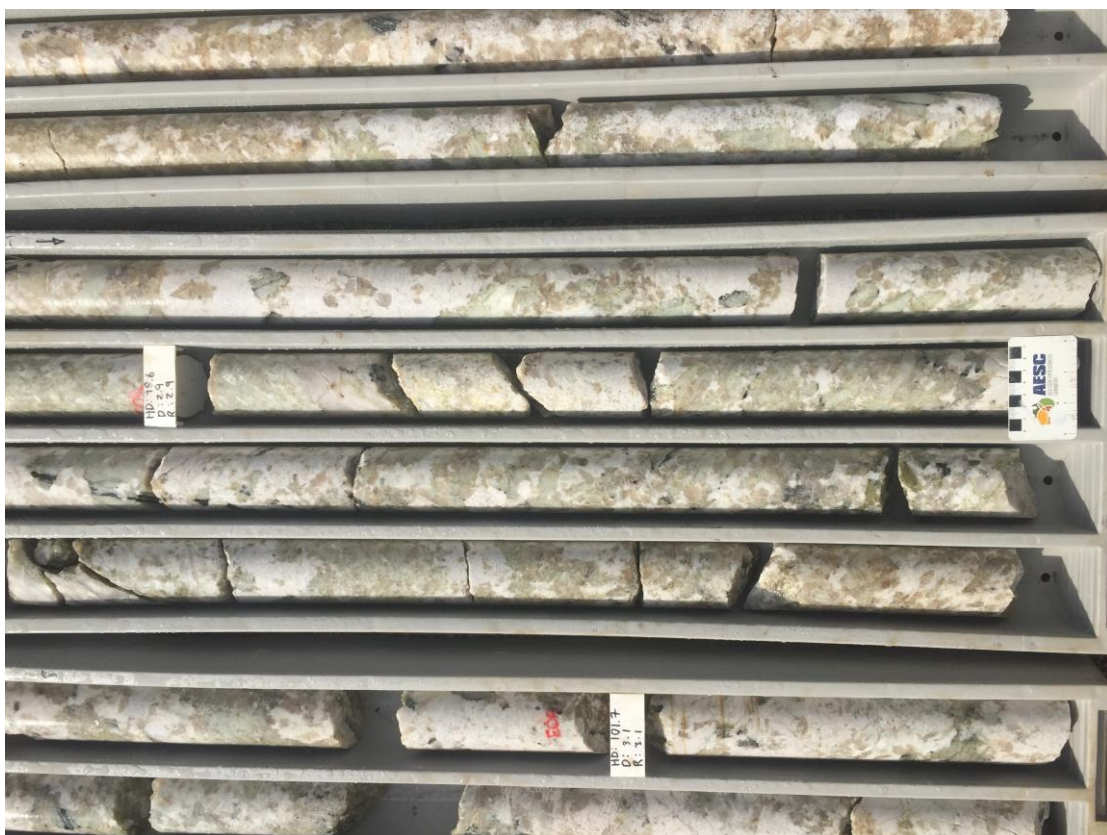
Figure 2. Large green spodumene crystals hosted by lighter coloured (white) feldspar and quartz. 95.2m – 103.1m FRDD001 (HQ), BP33 Prospect, Finniss Lithium Project NT.
