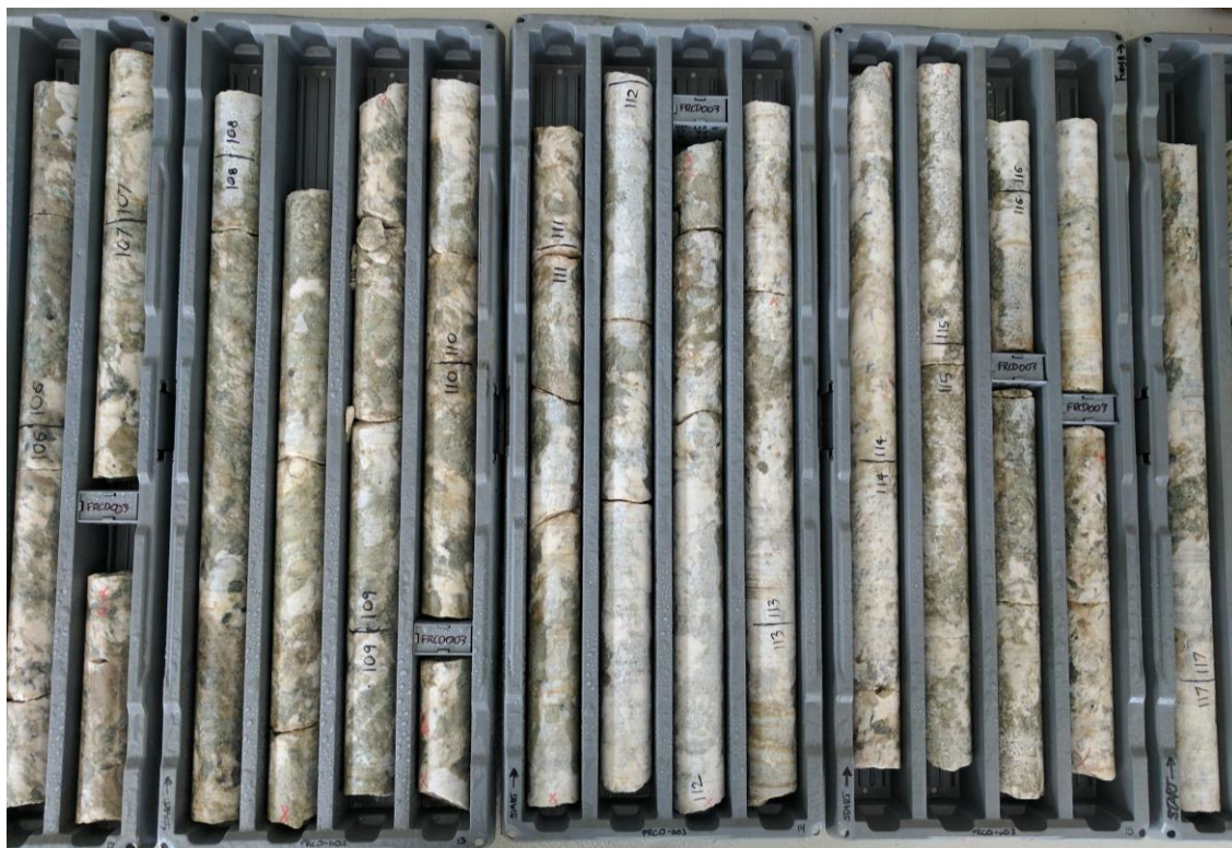
Figure 1. High grade spodumene intersection grading 2.03% Li 2 O (106m-116m). Large green spodumene crystals hosted by lighter coloured (white) feldspar and quartz. 105.5m – 117.7m FRDD003 (HQ) Grants Prospect, Finniss Lithium Project, NT.
