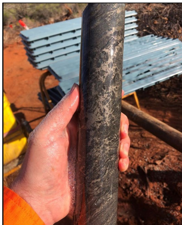
Figure 8 –Left- Wattle Dam East - Down Hole EM (DHEM) survey results. (Po – pyrrhotite). Right - Significant pyrrhotite mineralisation from 504.5m. NQ sized core.
