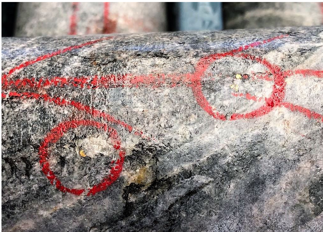
Figure 4. HQ Drill hole S05DD003 with visible gold at 80m depth. Visible gold does not characterise all mineralised intercepts at the S5 prospect. Red chinagraph lines are approximately 4mm wide, for scale.
