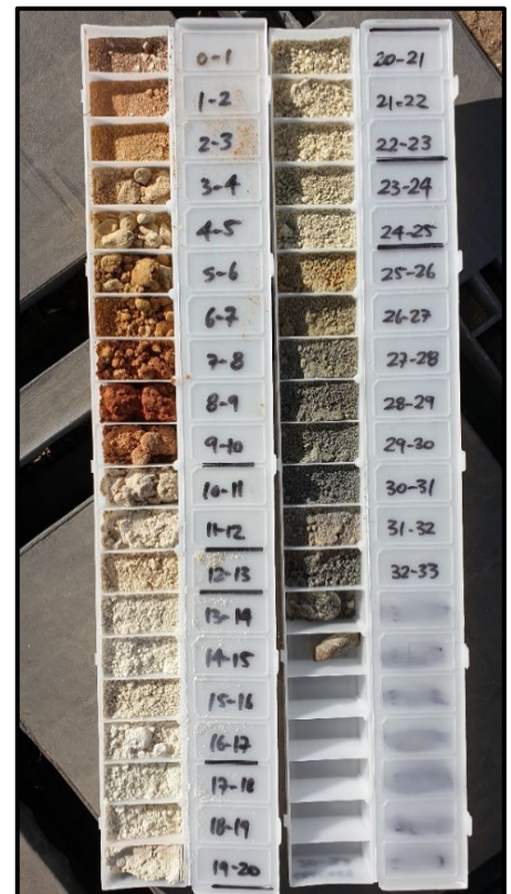
Figure 5: Oar's Gibraltar Project Drill cutting from GBAC069 showing white kaolinitic saprolite developed over gneissic basement material
