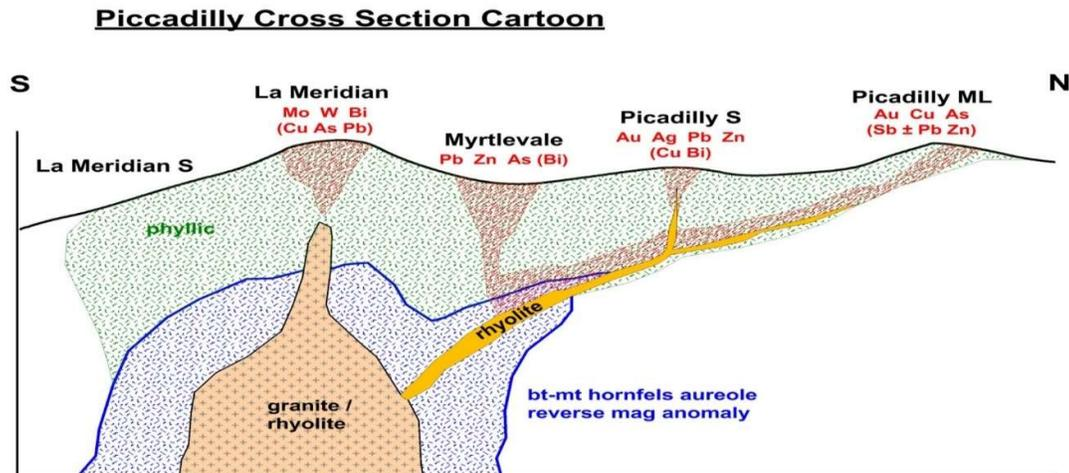
Figure 2 shows the Piccadilly Mining Lease to the north, with suggested mineralisation dipping to the south towards the intrusive related source. It is interesting to note that this figure was created some years ago by Dr Morrison, on behalf of Piccadilly Gold Mine Holdings Limited, and that the recent work completed by Cannindah Resources Limited has confirmed that the high-grade gold in the Mining Lease does indeed dip to the south towards this area.
