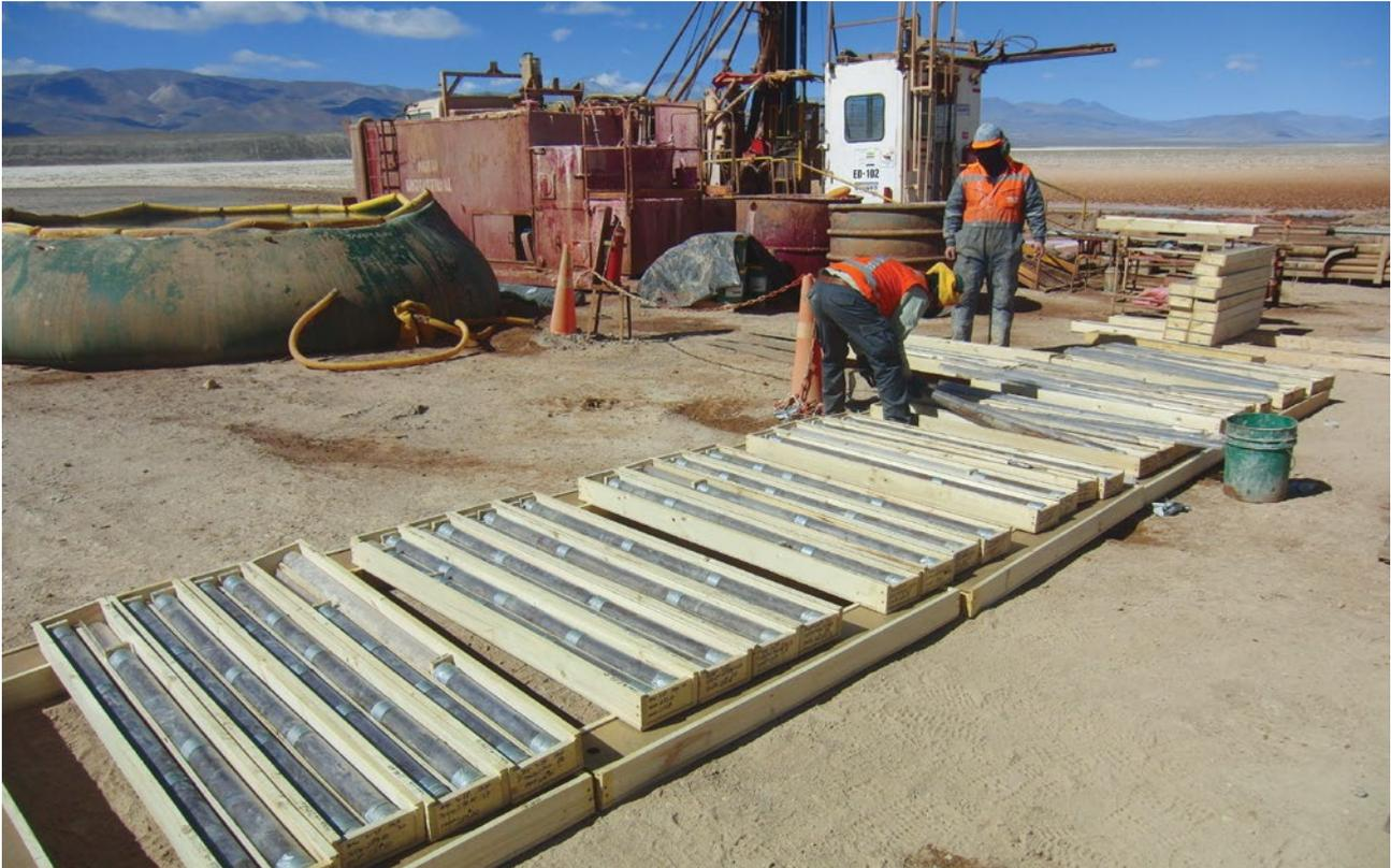
Figure 2: Exploration Diamond Core Holes - Major Drilling
