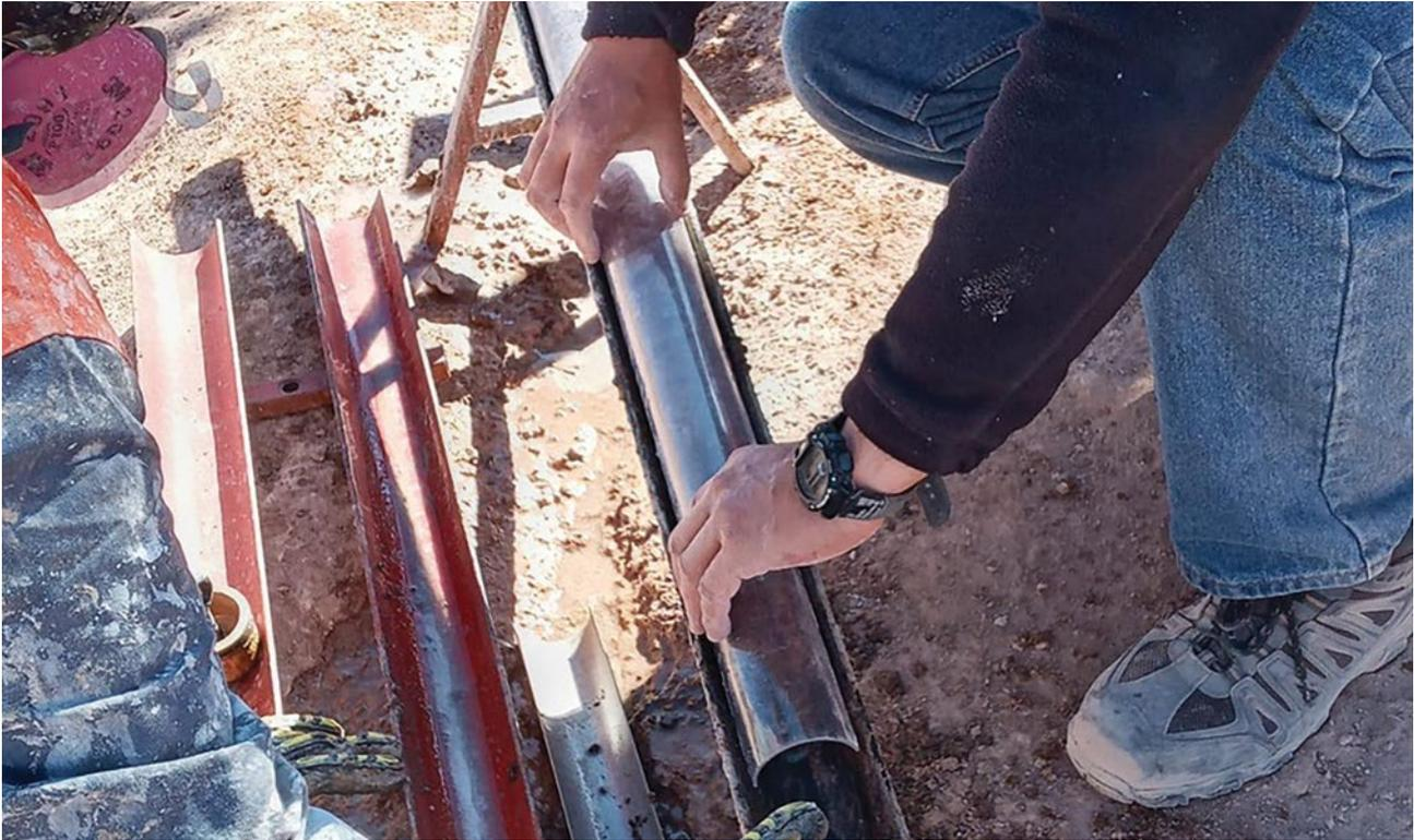
Figure 3: Exploration Diamond Core Holes – Drilling Samples
