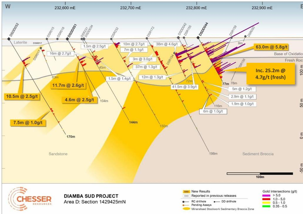
Figure 2: Section 1429425mN showing historical drilling, holes reported in this release, selected significant results<sup>2</sup> and interpreted geology.
