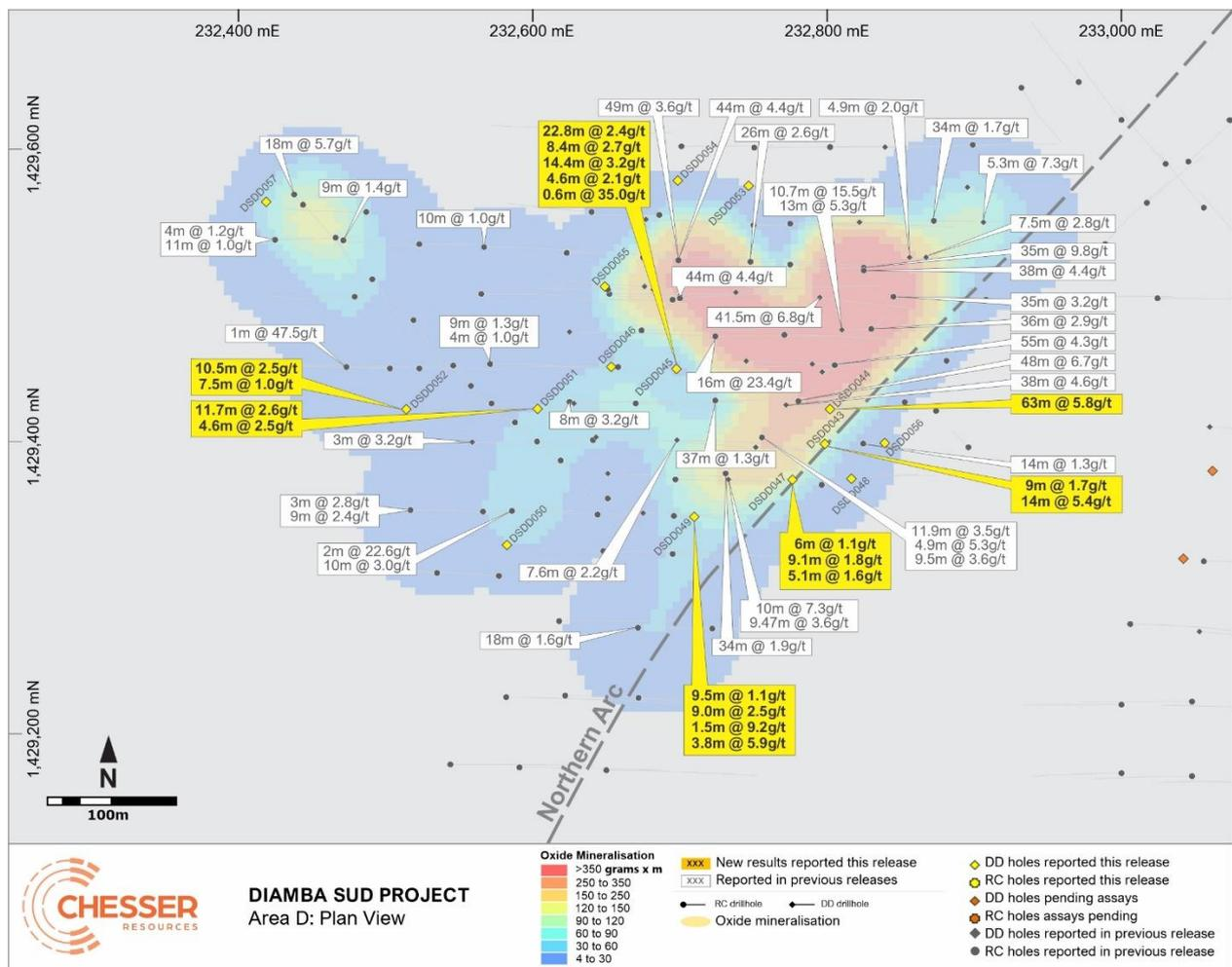
**Figure 1: Area D plan view showing historical drilling and holes reported in this release with selected significant results<sup>1</sup> and oxide mineralisation grade thickness contours.**
