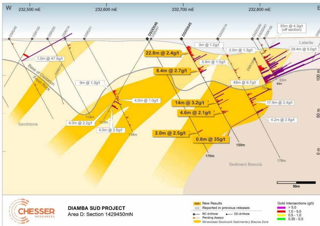
Figure 3: Section 1429450mN showing historical drilling, holes reported in this release, selected significant results<sup>3</sup> and interpreted geology.
