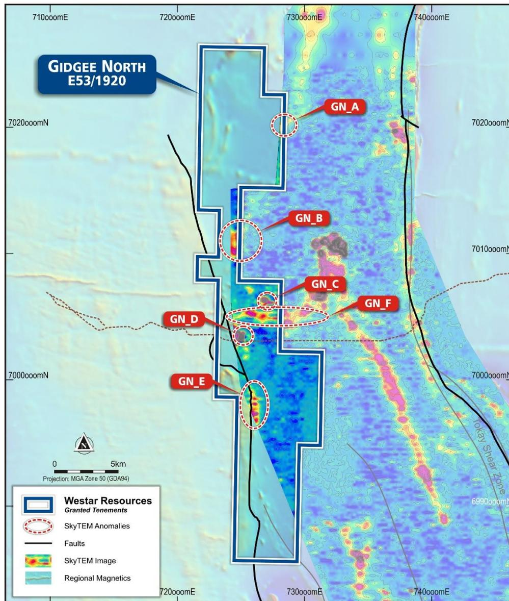
**Figure 1:** SkyTEM (high moment Ch35) shown with tenement boundary and anomalies identified.
