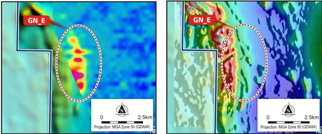
**Figure 4:** LHS shows SkyTEM (high moment Ch35) with anomaly GN\_E. RHS shows 80m magnetic TMI 1VD image with north shade at same scale. Refer to Figure 1 for map legend.
